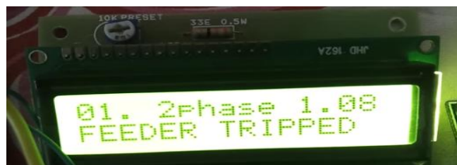
Fig-19 Display on LCD when the feeder tripped during 2-phase
